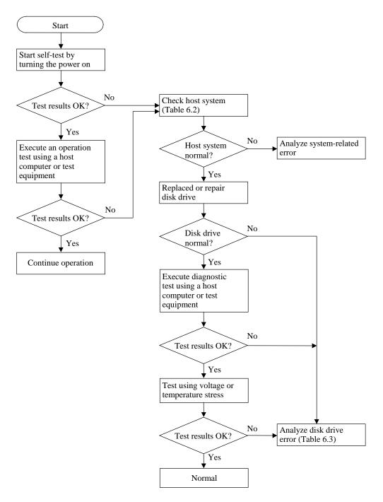
Figure 6.3 Test flowchart
